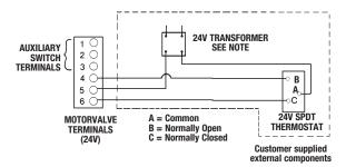
NOTE: 1/4" - 1/2" EMVII-6400SS-24-40 will operate with a 40 VA transformer. Thermostat must be capable of handling amp rating at stall.
