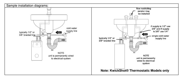
Open the hot water faucet and run water for a minimum of 60 seconds and until the flow is continuous and free of air pockets. Close the faucet and install the aerator (if supplied).
